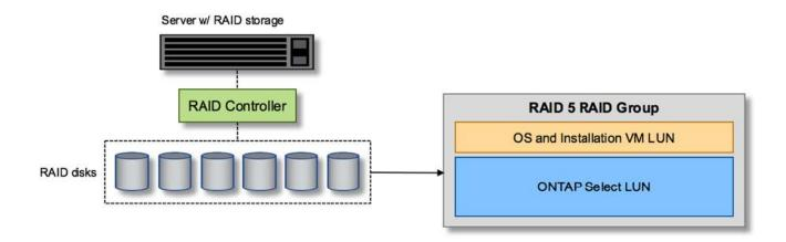
Provisioning the OS LUNs from the same RAID group as ONTAP Select allows the hypervisor OS (and any client VM that is also provisioned from that storage) to benefit from RAID protection. This configuration prevents a single-drive failure from bringing down the entire system.
