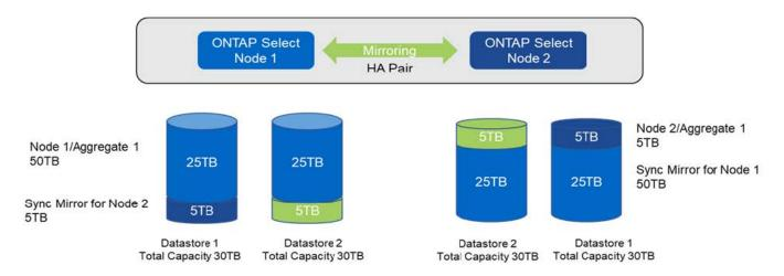
The maximum VMDK size used during capacity add operations is 16TB. The maximum VMDK size used during cluster create operations continues to be 8TB. ONTAP Deploy creates correctly sized VMDKs depending on your configuration (a single-node or multinode cluster) and the amount of capacity being added. However, the maximum size of each VMDK should not exceed 8TB during the cluster create operations and 16TB during the storage-add operations.
