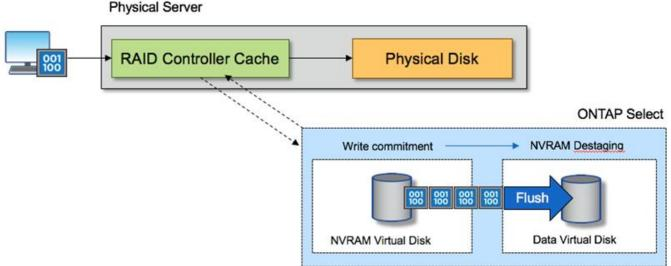
The NVRAM partition is separated on its own VMDK. That VMDK is attached using the vNVME driver available in ESX versions of 6.5 or later. This change is most significant for ONTAP Select installations with software RAID, which do not benefit from the RAID controller cache.
