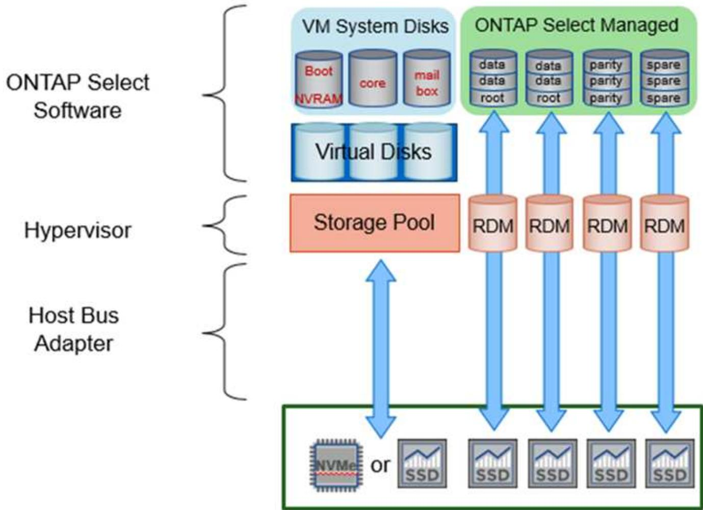
The system disks (VMDKs) reside in the same datastore and on the same physical disk. The virtual NVRAM disk requires a fast and durable media. Therefore, only NVMe and SSD-type datastores are supported.
