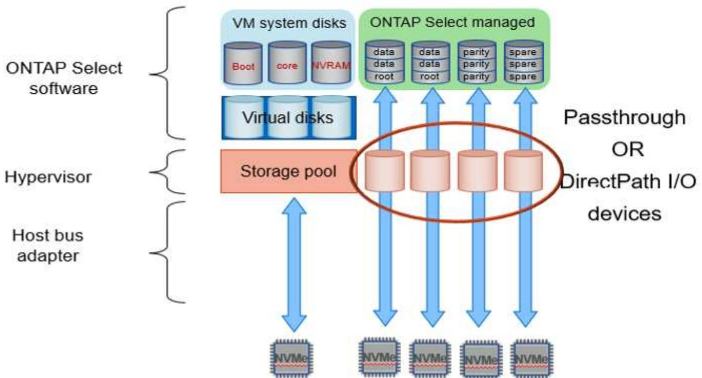
The system disks (VMDKs) reside in the same datastore and on the same physical disk. The virtual NVRAM disk requires a fast and durable media. Therefore, only NVMe and SSD-type datastores are supported. When using NVMe drives for data, the system disk should also be an NVMe device for performance reasons. A good candidate for the system disk in an all NVMe configuration is an INTEL Optane card.
