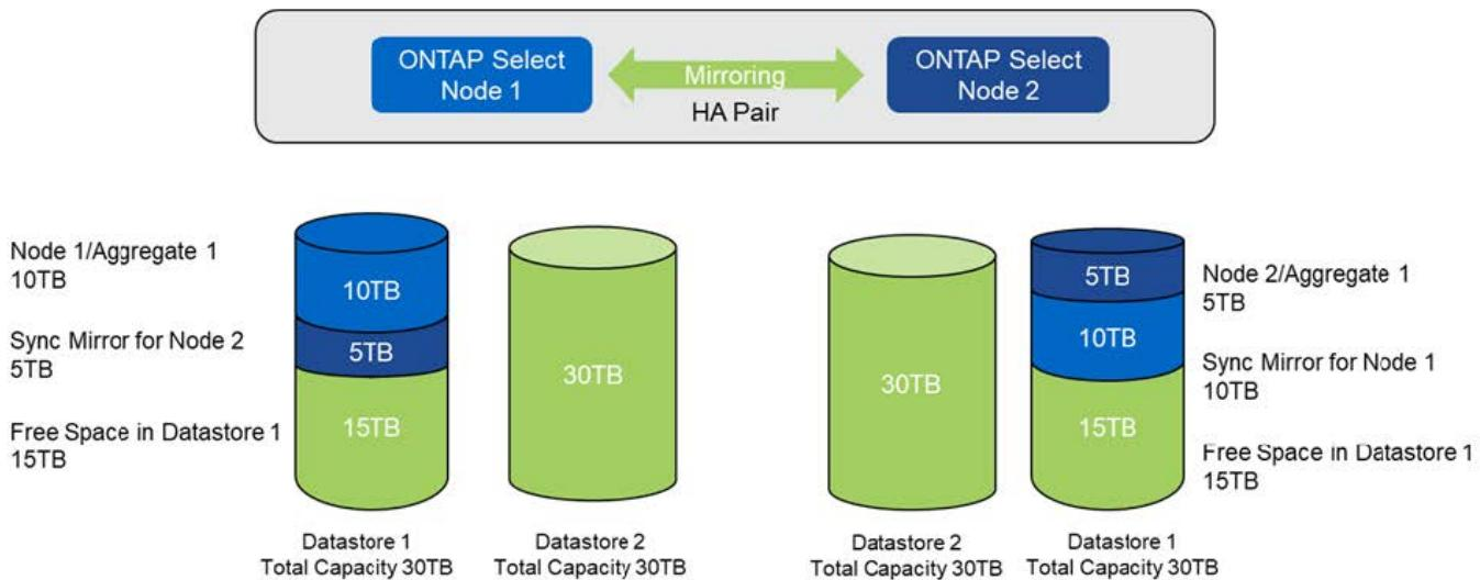
Two additional storage-add operations on node 1 consume the rest of datastore 1 and a part of datastore 2 (using the capacity cap). The first storage-add operation consumes the 15TB of free space left in datastore 1. The following figure shows the result of the second storage-add operation. At this point, node 1 has 50TB of active data under management, while node 2 has the original 5TB.
