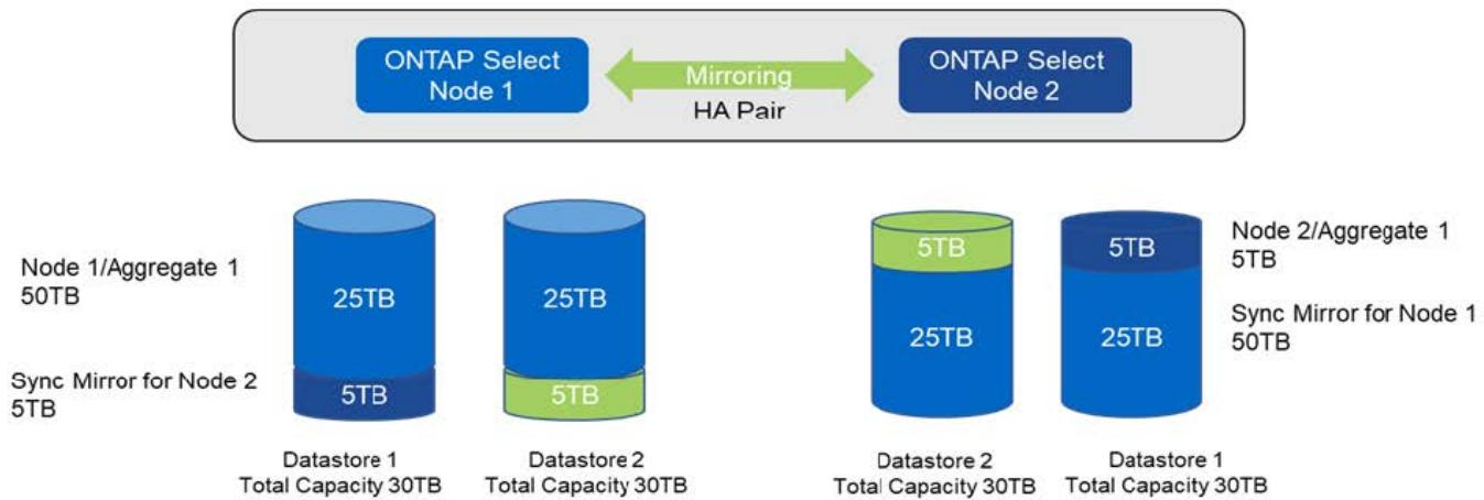
The maximum VMDK size used during capacity add operations is 16TB. The maximum VMDK size used during cluster create operations continues to be 8TB. ONTAP Deploy creates correctly sized VMDKs depending on your configuration (a single-node or multinode cluster) and the amount of capacity being added. However, the maximum size of each VMDK should not exceed 8TB during the cluster create operations and 16TB during the storage-add operations.
