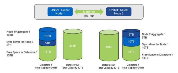
Two additional storage-add operations on node 1 consume the rest of datastore 1 and a part of datastore 2 (using the capacity cap). The first storage-add operation consumes the 15TB of free space left in datastore 1. The following figure shows the result of the second storage-add operation. At this point, node 1 has 50TB of active data under management, while node 2 has the original 5TB.
