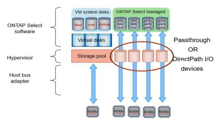
The system disks (VMDKs) reside in the same datastore and on the same physical disk. The virtual NVRAM disk requires a fast and durable media. Therefore, only NVMe and SSD-type datastores are supported. When using NVMe drives for data, the system disk should also be an NVMe device for performance reasons. A good candidate for the system disk in an all NVMe configuration is an INTEL Optane card.
