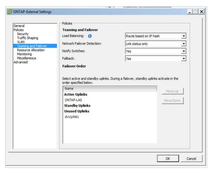
Internal port group configurations using a distributed vSwitch with LACP enabled
