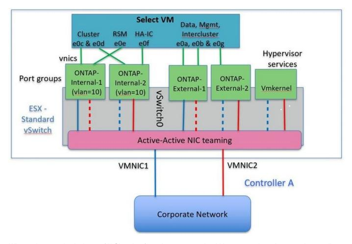
When using two physical ports (10Gb or less), each port group should have an active adapter and a standby adapter configured opposite to each other. The internal network is only present for multinode ONTAP Select clusters. For single-node clusters, both adapters can be configured as active in the external port group.
