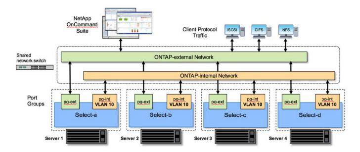
Each ONTAP Select VM contains seven virtual network adapters presented to ONTAP as a set of seven network ports, e0a through e0g. Although ONTAP treats these adapters as physical NICs, they are in fact virtual and map to a set of physical interfaces through a virtualized network layer. As a result, each hosting server does not require six physical network ports.
