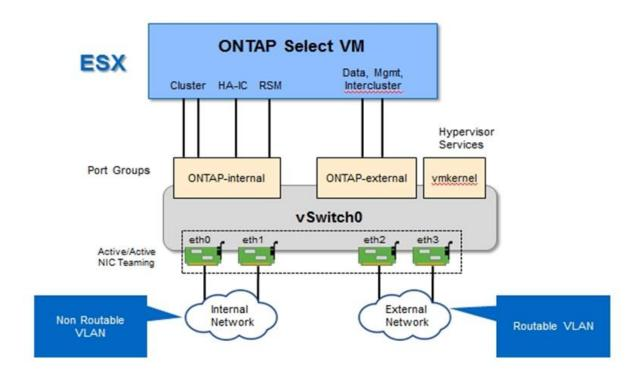
Segregating internal and external traffic across different physical NICs prevents latencies from being introduced into the system due to insufficient access to network resources. Additionally, aggregation through NIC teaming makes sure that failure of a single network adapter does not prevent the ONTAP Select cluster node from accessing the respective network.
