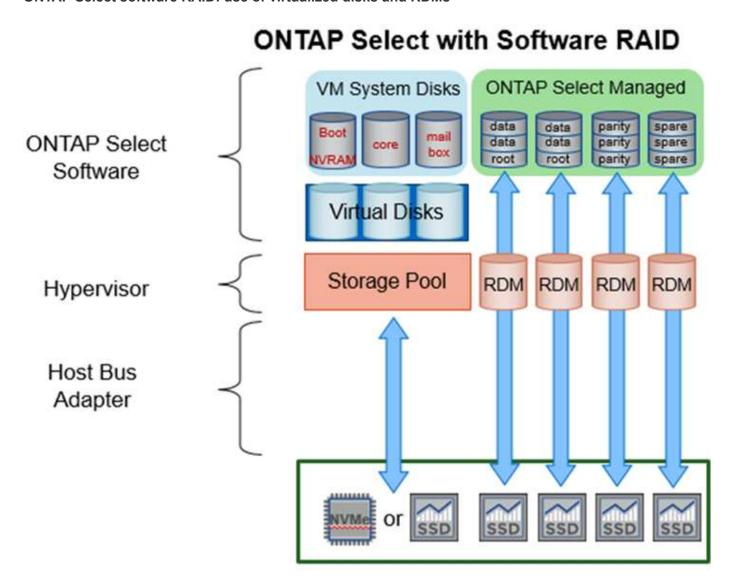
The system disks (VMDKs) reside in the same datastore and on the same physical disk. The virtual NVRAM disk requires a fast and durable media. Therefore, only NVMe and SSD-type datastores are supported.
