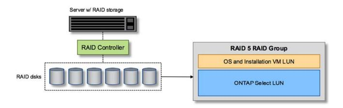
Provisioning the OS LUNs from the same RAID group as ONTAP Select allows the hypervisor OS (and any client VM that is also provisioned from that storage) to benefit from RAID protection. This configuration prevents a single-drive failure from bringing down the entire system.
