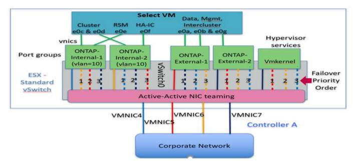
The order of the ports in the standby list is important. The following table provides an example of the physical port distribution across the four port groups.
