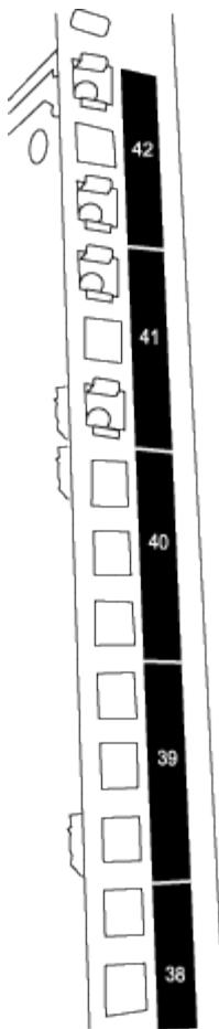
The two 3232C switches will always be mounted in the top 2U of the cabinet RU41 and 42.
