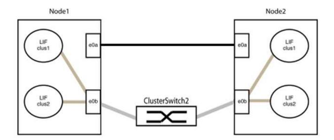
9. The switchless cluster network option transitions from false to true. This might take up to 45 seconds. Confirm that the switchless option is set to true:
