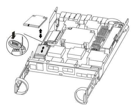
3. Press the blue button on the boot media housing to release the boot media from its housing, and then gently pull it straight out of the boot media socket.
