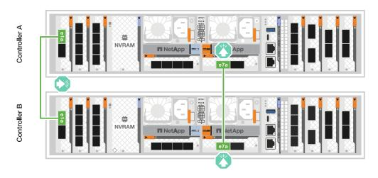
2. Cable the Ethernet module ports to your host network.
