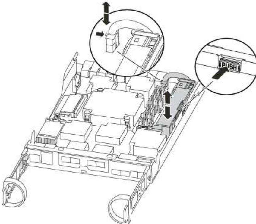
4. Locate the battery plug and squeeze the clip on the face of the battery plug to release the plug from the socket, and then unplug the battery cable from the socket.
