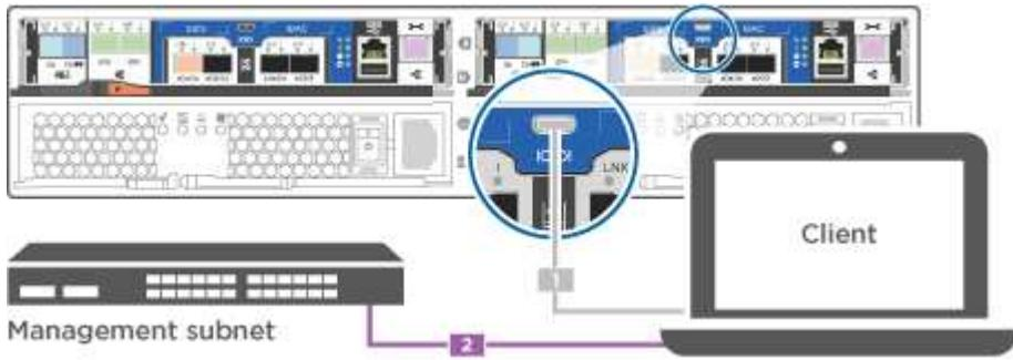
d. Assign a TCP/IP address to the laptop or console, using one that is on the management subnet.
