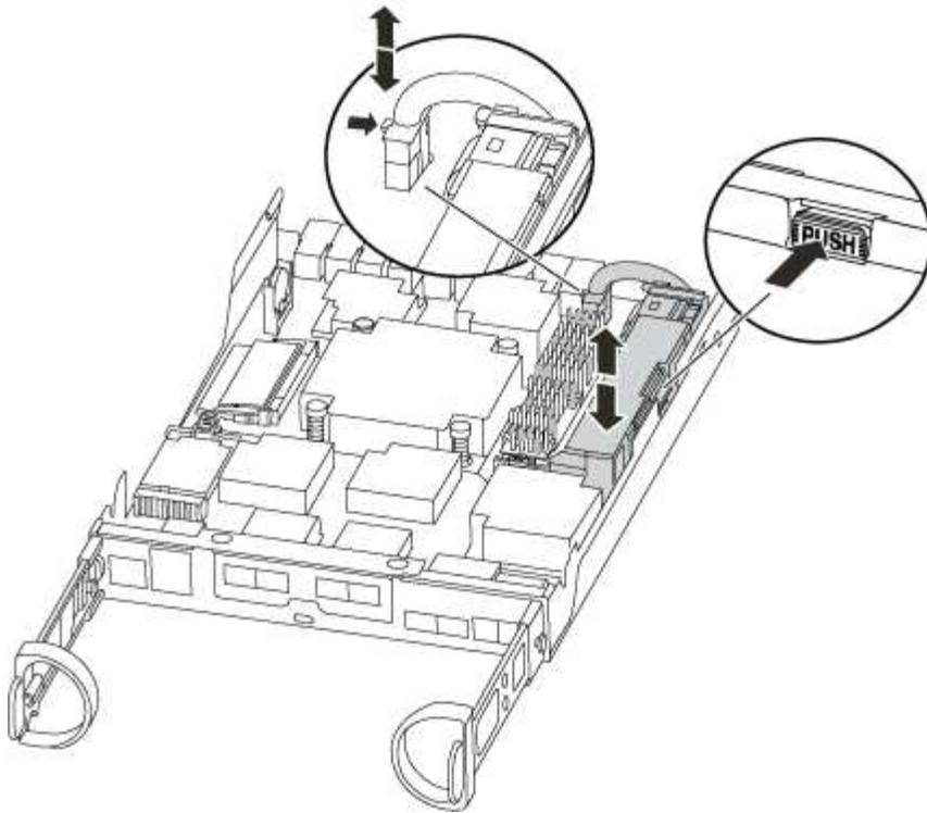
3. Locate the battery plug and squeeze the clip on the face of the battery plug to release the plug from the socket, and then unplug the battery cable from the socket.
