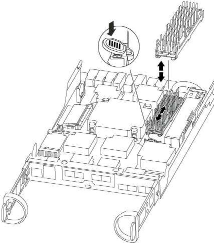
2. Gently pull the caching module straight out of the housing.
