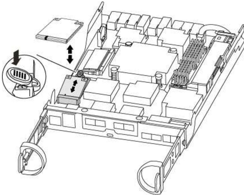
2. Press the blue button on the boot media housing to release the boot media from its housing, and then gently pull it straight out of the boot media socket.
