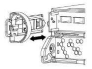
3. Squeeze the latch on the cam handle until it releases, open the cam handle fully to release the controller module from the midplane, and then, using two hands, pull the controller module out of the chassis.
