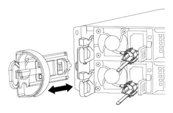
Leave the cables in the cable management device so that when you reinstall the cable management device, the cables are organized.
