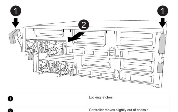
6. Slide the controller module out of the chassis.
