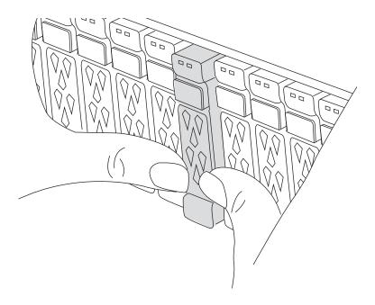
2. Check the amber NVRAM that status LED located in slot 4/5 on the back of the impaired controller module is off. Look for the NV icon.
