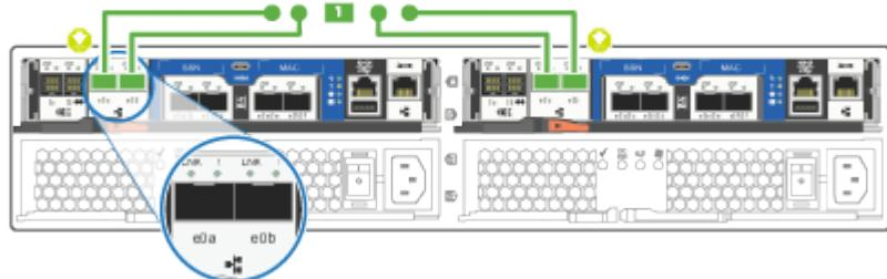
2. Cable the controllers to either a UTA2 data network or an Ethernet network.
