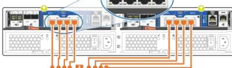
3. Cable the e0M ports to the management network switches with the RJ45 cables.
