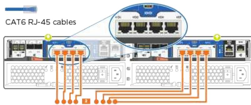
3. Cable the e0M ports to the management network switches with the RJ45 cables.
