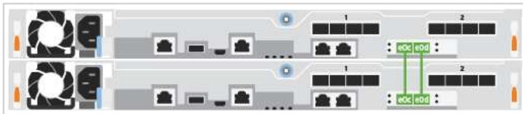
2. Cable the wrench ports to the management network switches with the RJ45 cables.
