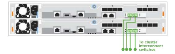
2. Cable the wrench ports to the management network switches with the RJ45 cables.
