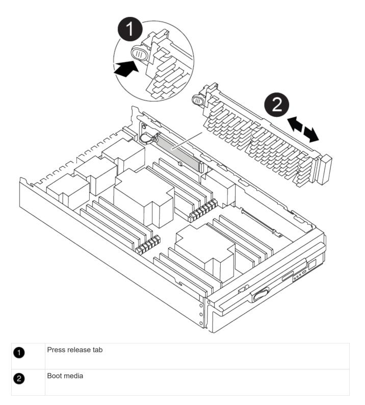
2. Press the blue button on the boot media housing to release the boot media from its housing, and then gently pull it straight out of the boot media socket.
