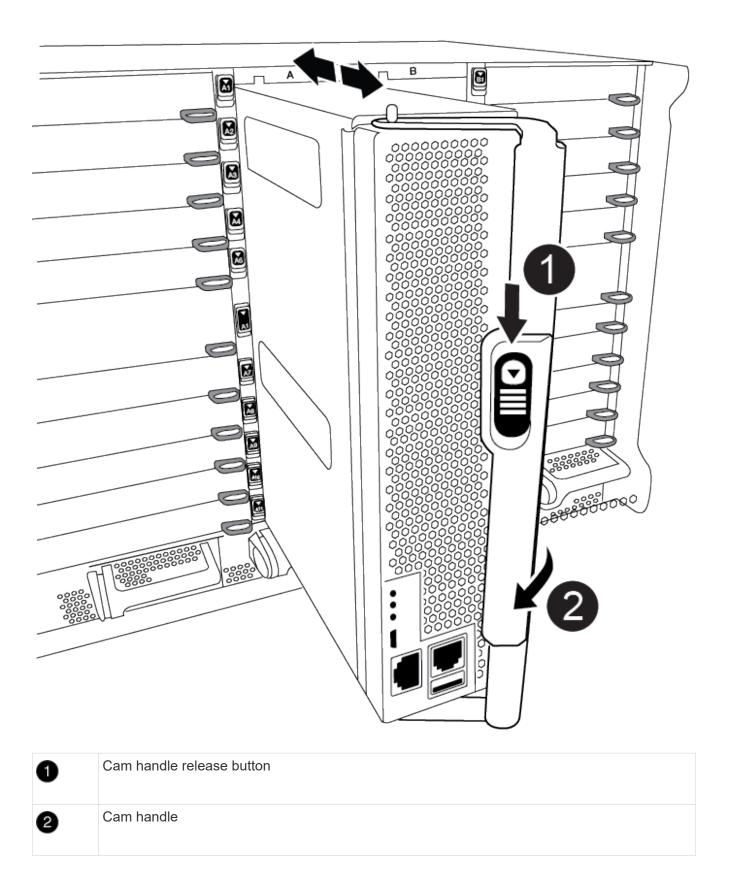
4. Rotate the cam handle so that it completely disengages the controller module from the chassis, and then slide the controller module out of the chassis.
