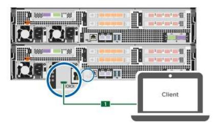
c. Connect the laptop or console to the switch on the management subnet.
