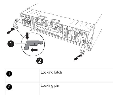
8. Slide the controller module out of the chassis and place it on a flat, stable surface.
