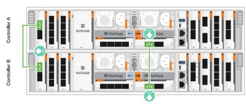
2. Connect the Ethernet module ports to your host network.
