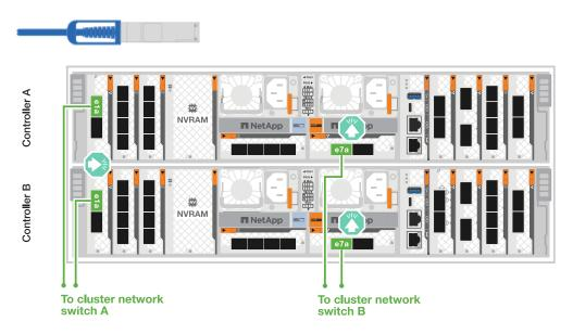
2. Connect the Ethernet module ports to your host network.
