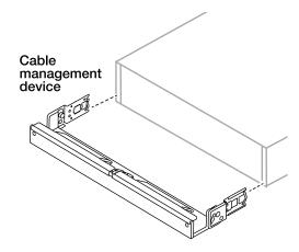
5. Attach the bezel to the front of the storage system.
