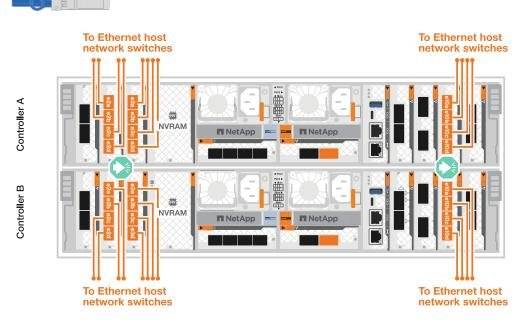
3. Use the 1000BASE-T RJ-45 cables to connect the controller management (wrench) ports to the management network switches.
