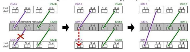
Verify that you bypassed the disk shelves you are removing and reestablished the path A (IOM A) stack connections correctly: storage disk show -port
