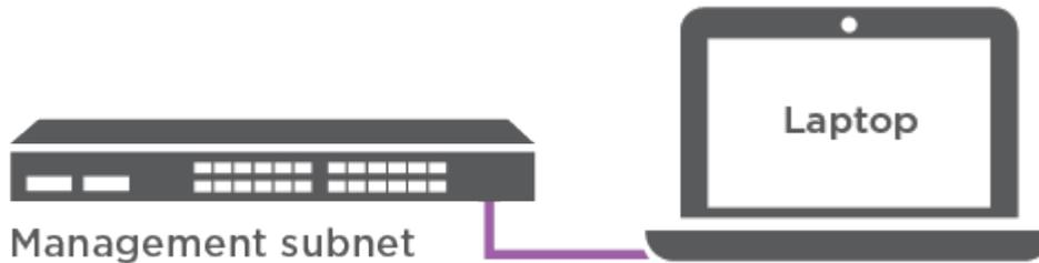
c. Assign a TCP/IP address to the laptop or console, using one that is on the management subnet.
