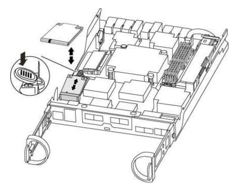
3. Press the blue button on the boot media housing to release the boot media from its housing, and then
