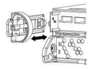
4. Squeeze the latch on the cam handle until it releases, open the cam handle fully to release the controller module from the midplane, and then, using two hands, pull the controller module out of the chassis.
