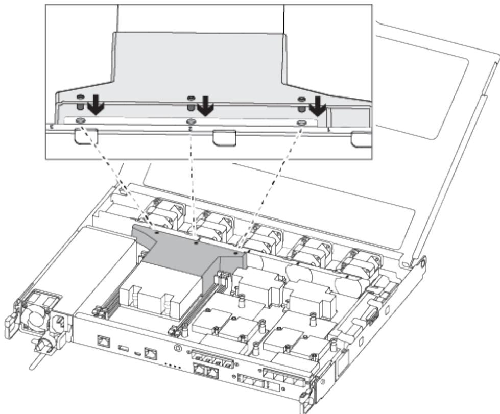
f. Close the controller module cover and tighten the thumbscrew.
