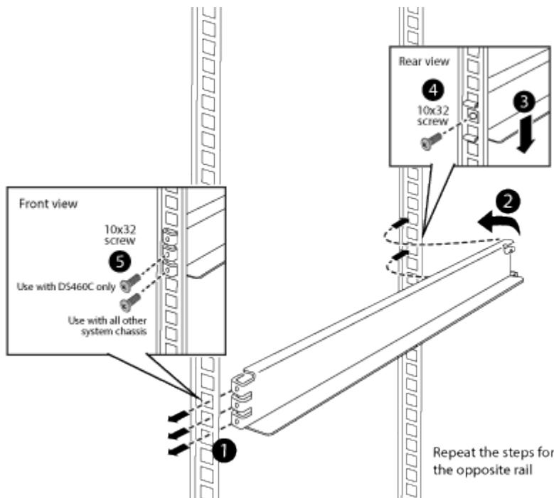
3. If your equipment mounting flanges extend beyond the screw holes in the support rail, install cage nuts above the support rail, where needed.
