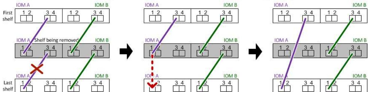
6. Verify that you bypassed the disk shelves you are removing and reestablished the path A (IOM A) stack connections correctly: `storage disk show -port`
