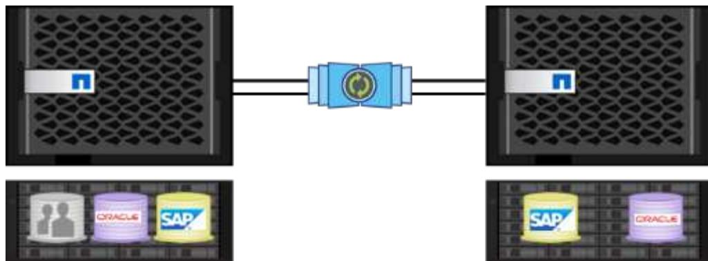
MetroCluster immediately duplicates all your mission-critical data on a transaction-by-transaction basis, providing uninterrupted access to your applications and data. Unlike standard data replication solutions, MetroCluster works seamlessly with your host environment to provide continuous data availability while eliminating the need to create and maintain complicated failover scripts.
