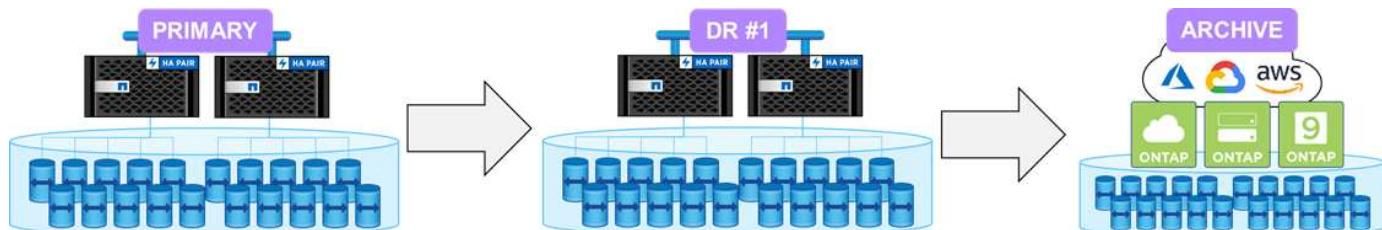
SnapMirror fan-out can replicate from a source volume to multiple destination volumes. So site A can replicate a source FlexGroup to sites B and C (on-prem or cloud). This offers more flexibility and resiliency in data protection configurations.
