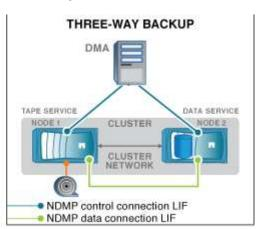
Using the affinity information about volumes and tape devices, the DMA (backup application) performs a local NDMP backup on the volume and tape device located on Node 1 in the cluster. If the volume moves from Node 1 to Node 2, affinity information about the volume and tape device changes. Hence, for a subsequent backup the DMA performs a three-way NDMP backup operation. This ensures continuity of the backup policy for the volume irrespective of the node to which the volume is moved to.
