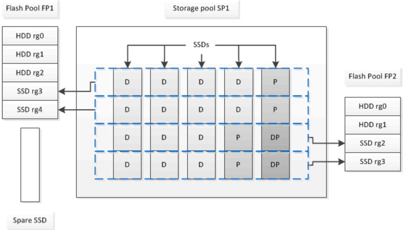
Storage pool SP1 is composed of five SSDs and a hot spare SSD. Two of the storage pool's allocation units are allocated to Flash Pool FP1, and two are allocated to Flash Pool FP2. FP1 has a cache RAID type of RAID4. Therefore, the allocation units provided to FP1 contain only one partition designated for parity. FP2 has a cache RAID type of RAID-DP. Therefore, the allocation units provided to FP2 include a parity partition and a double-parity partition.
