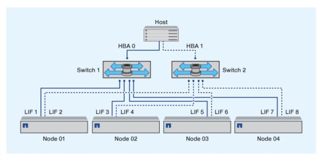
The host operating system and multipathing software have to support the number of paths that is being used to access the LUNs on the nodes.
