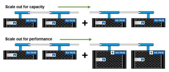
You can scale out for capacity by adding nodes with like controller models, or for performance by adding nodes with higher-end storage arrays, all while clients and hosts continue to access data.
