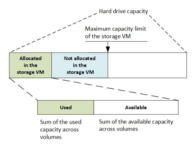
Beginning with ONTAP 9.13.1, cluster administrators can enable a maximum capacity limit for a storage VM. However, storage limits cannot be set for a storage VM that contains volumes that are for data protection, in a SnapMirror relationship, or in a MetroCluster configuration. Also, quotas cannot be configured to exceed the maximum capacity of a storage VM.
