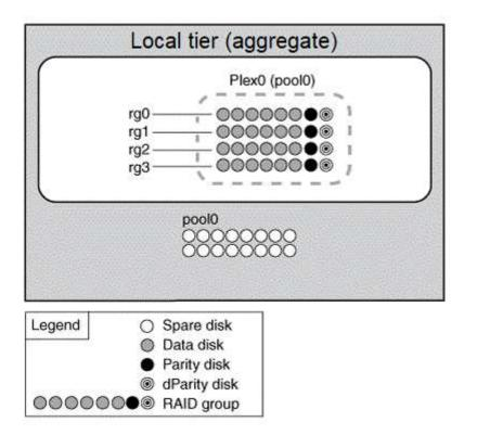
The following diagram shows an unmirrored local tier with array LUNs, with its one plex. It has two RAID groups, rg0 and rg1. All array LUNs used by the local tier come from the same pool, "pool0".
