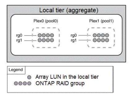
It's recommended you maintain at least 20% free space for mirrored aggregates for optimal storage performance and availability. Although the recommendation is 10% for non-mirrored aggregates, the additional 10% of space may be used by the filesystem to absorb incremental changes. Incremental changes increase space utilization for mirrored aggregates due to ONTAP's copy-on-write Snapshot-based architecture. Failure to adhere to these best practices may have a negative impact on performance.
