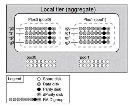
The following diagram shows an local tier composed of array LUNs with the SyncMirror functionality enabled and implemented. A second plex has been created for the local tier, "plex1". Plex1 is a copy of plex0, and the RAID groups are also identical.
