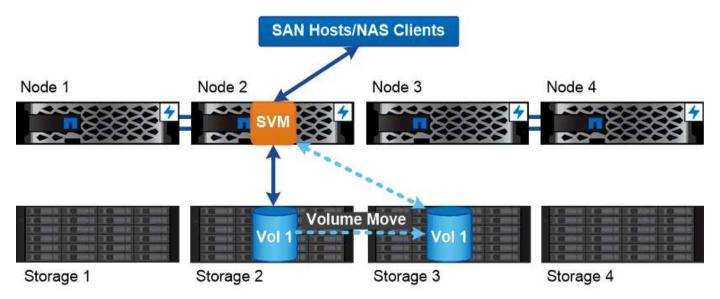
Data accessed through an SVM is not bound to a physical storage location. You can move a volume without disrupting data service.
