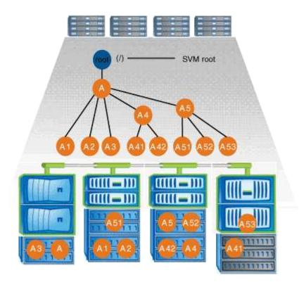
For example, a typical volume junction configuration with the above namespace architecture might look like the following configuration, where all volumes are junctioned below the single insertion point, which is a directory named "data":
