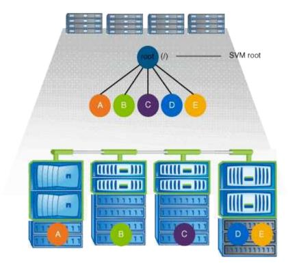
For example, a typical volume junction configuration with the above namespace architecture might look like the following configuration, where there are five insertion points to the root volume of the SVM, with each insertion point representing a path to one volume.
