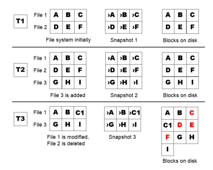
A Snapshot copy consumes disk space only when blocks in the active file system are modified or deleted.
