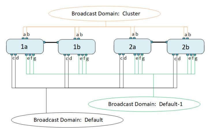
A failover group of the same name and with the same network ports as each of the broadcast domains is created automatically. This failover group is automatically managed by the system, meaning that as ports are added or removed from the broadcast domain, they are automatically added or removed from this failover group.
