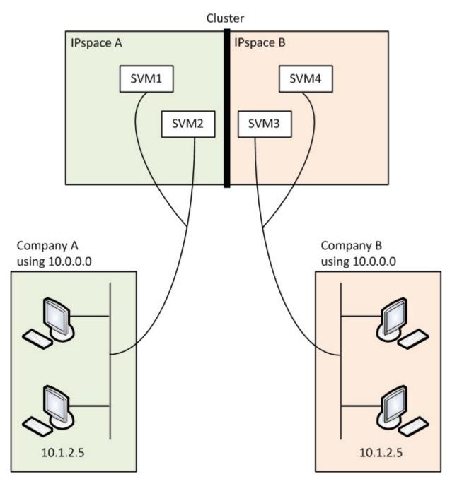
Additionally, the IP addresses referred to by the various configuration files, such as the /etc/ hosts file, the /etc/hosts.equiv file, and the /etc/rc file, are relative to that IPspace. Therefore, the IPspaces enable the SSP to configure the same IP address for the configuration and authentication data for multiple SVMs, without conflict.
