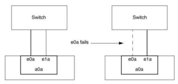
To accomplish single-mode functionality, the recommended approach is to instead use failover groups. By using a failover group, the second port can still be used for other LIFs and need not remain unused. Additionally, failover groups can span more than two ports and can span ports on multiple nodes.
