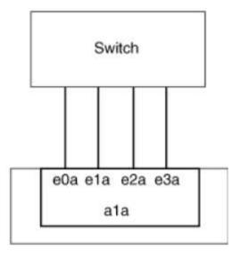
Several technologies exist that enable traffic in a single aggregated link to be distributed across multiple physical switches. The technologies used to enable this capability vary among networking products. Static multimode interface groups in ONTAP conform to the IEEE 802.3 standards. If a particular multiple switch link aggregation technology is said to interoperate with or conform to the IEEE 802.3 standards, it should operate with ONTAP.
