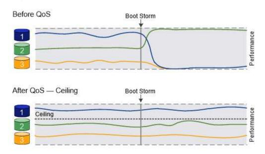
The throughput ceiling for workload 2 ensures that it does not "bully" workloads 1 and 3.
