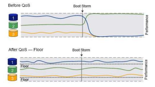
The throughput floors for workload 1 and workload 3 ensure that they meet minimum throughput targets, regardless of demand by workload 2.
