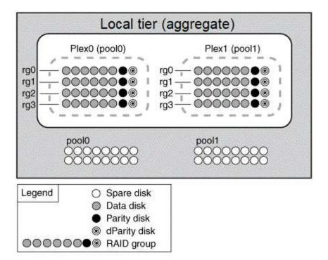
The following diagram shows an local tier composed of array LUNs with the SyncMirror functionality enabled and implemented. A second plex has been created for the local tier, "plex1". Plex1 is a copy of plex0, and the RAID groups are also identical.
