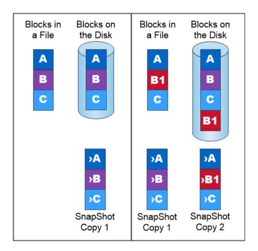
A Snapshot copy records only changes to the active file system since the last Snapshot copy.
