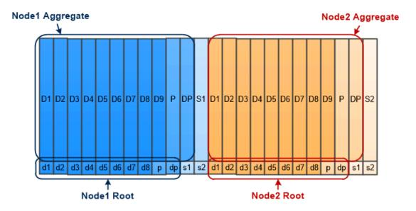
Root-data partitioning creates one small partition on each disk as the root partition and one large partition on each disk for data.
