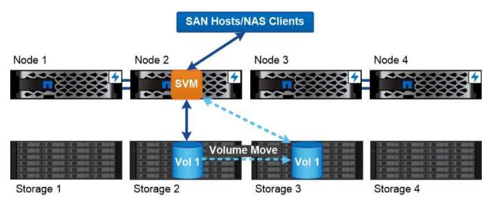
Data accessed through an SVM is not bound to a physical storage location. You can move a volume without disrupting data service.
