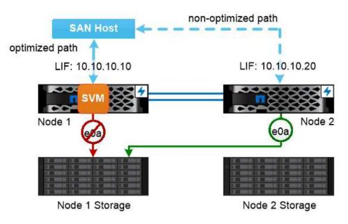
A SAN host uses multipathing technology to reroute traffic to a surviving LIF after a link failure.
