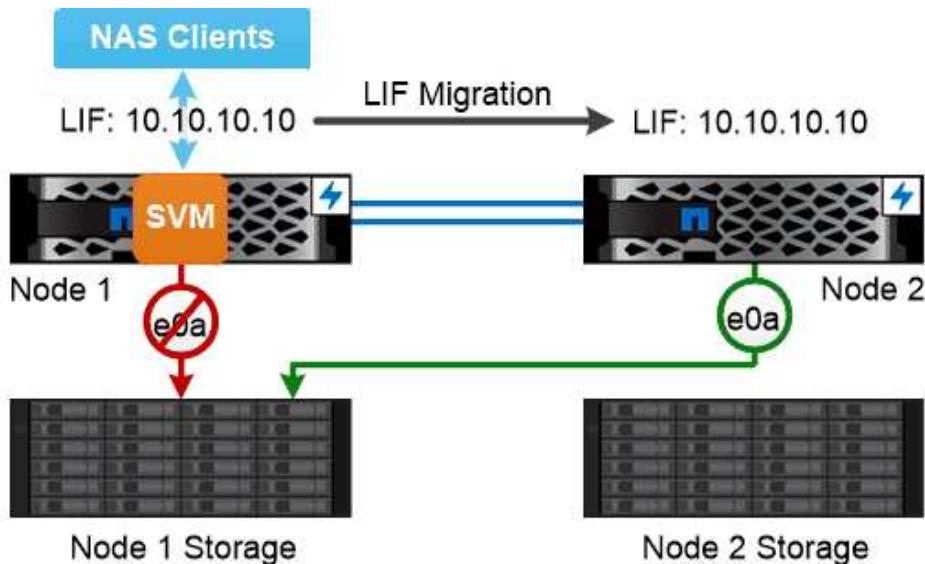
*A NAS LIF automatically migrates to a surviving network port after a link failure on its current port.*
