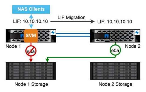
A NAS LIF automatically migrates to a surviving network port after a link failure on its current port.
