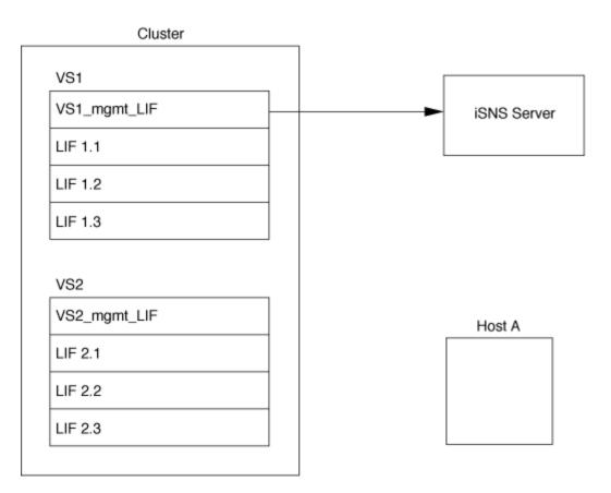
In the next example, after the iSNS server completes the registration with the target, Host A can discover all the LIFs for "VS1" through the iSNS server as indicated in Step 1. After Host A completes the discovery of the LIFs for "VS1", Host A can establish a connection with any of the LIFs in "VS1" as shown in Step 2. Host A is not aware of any of the LIFs in "VS2" until management LIF "VS2\_mgmt\_LIF" for "VS2" registers with the iSNS server.
