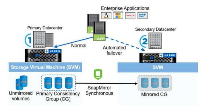
The diagram shows an enterprise application that is hosted on an storage VM (SVM) at the primary data center. The SVM contains five volumes, three of which are part of a consistency group. The three volumes in the consistency group are mirrored to a secondary data center. In normal circumstances, all write operations are performed to the primary data center; in effect, this data center serves as the source for I/O operations, while the secondary data center serves as a destination.
