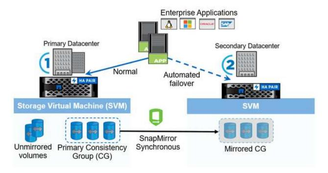
In section one of the diagram, an application is deployed on a SVM in the primary data center. The volumes that have been added to the primary consistency group are protected with SM-BC and are mirrored to secondary consistency group at a secondary data center. The volumes in the primary consistency group will failover to the mirrored consistency group in the event of a disruption. Volumes not in a mirrored consistency group are not served in the event of a failover.
