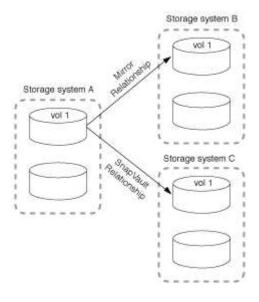
Beginning with ONTAP 9.5, you can have fan-out deployments with SnapMirror Synchronous relationships;
