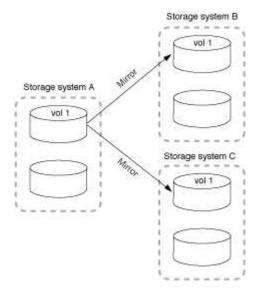
A mirror-vault fan-out deployment consists of a source volume that has a mirror relationship to a secondary volume and a SnapVault relationship to a different secondary volume.
