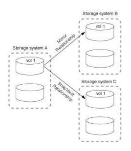
Beginning with ONTAP 9.5, you can have fan-out deployments with SnapMirror synchronous relationships; however, only one relationship in the fan-out configuration can be a SnapMirror synchronous relationship, all the other relationships from the source volume must be SnapMirror asynchronous relationships.
