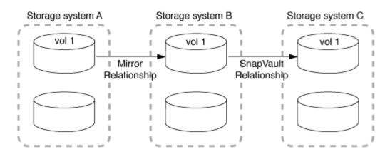
Vault-mirror and, beginning with ONTAP 9.2, vault-vault cascade deployments are also supported:
