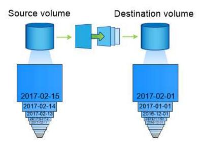
A SnapVault data protection relationship typically retains point-in-time Snapshot copies created over a longer period than the Snapshot copies on the source volume.
