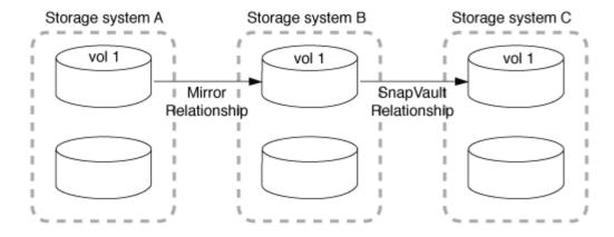
Vault-mirror and, beginning with ONTAP 9.2, vault-vault cascade deployments are also supported:
