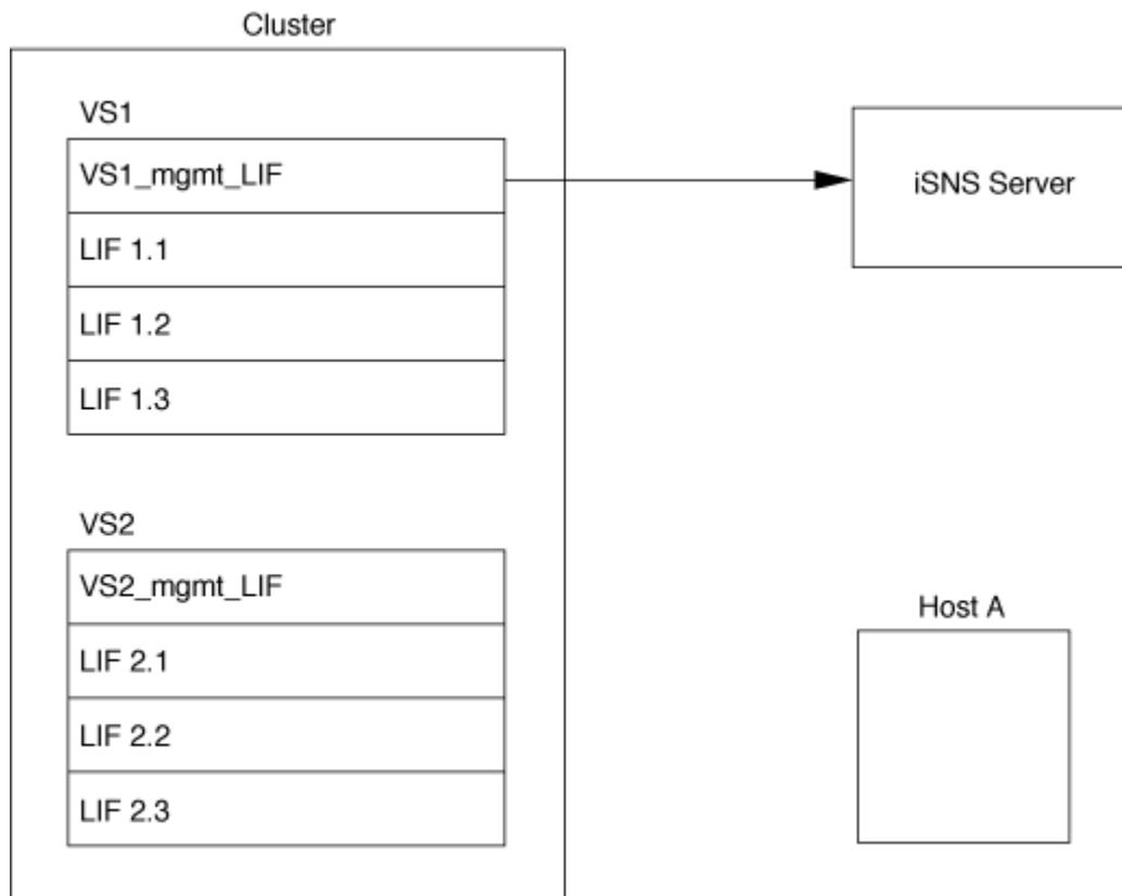
In the next example, after the iSNS server completes the registration with the target, Host A can discover all the LIFs for “VS1” through the iSNS server as indicated in Step 1. After Host A completes the discovery of the LIFs for “VS1”, Host A can establish a connection with any of the LIFs in “VS1” as shown in Step 2. Host A is
