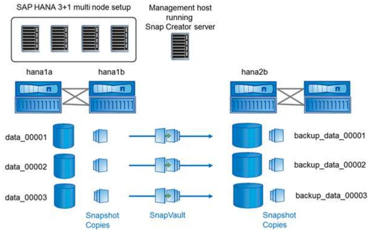
**i** All volumes that need to be backed up must be created on the secondary storage controller. In this example, the volumes backup\_data\_00001, backup\_data\_00002, and backup\_data\_00003 are created on the secondary storage controller.
