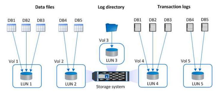
The following graphic shows how you can configure the storage layout for large databases on VMDKs:
