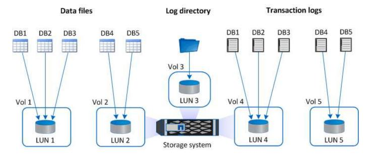
The following graphic shows how you can configure the storage layout for large databases on VMDKs:
