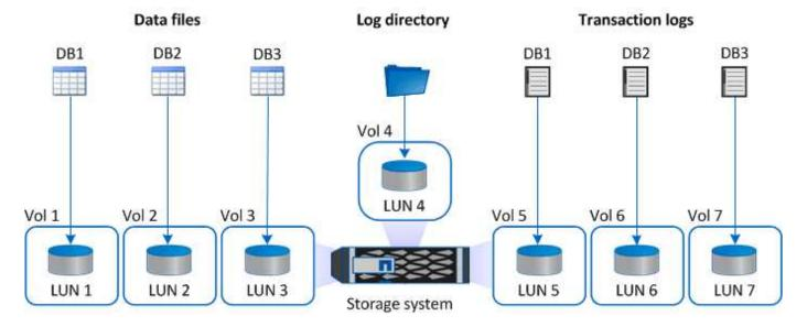
The following graphic shows how you can configure the storage layout for medium or small databases on LUNs:
