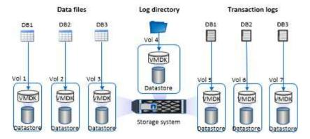
The following graphic shows how you can configure the storage layout for medium or small databases on VMDKs:
