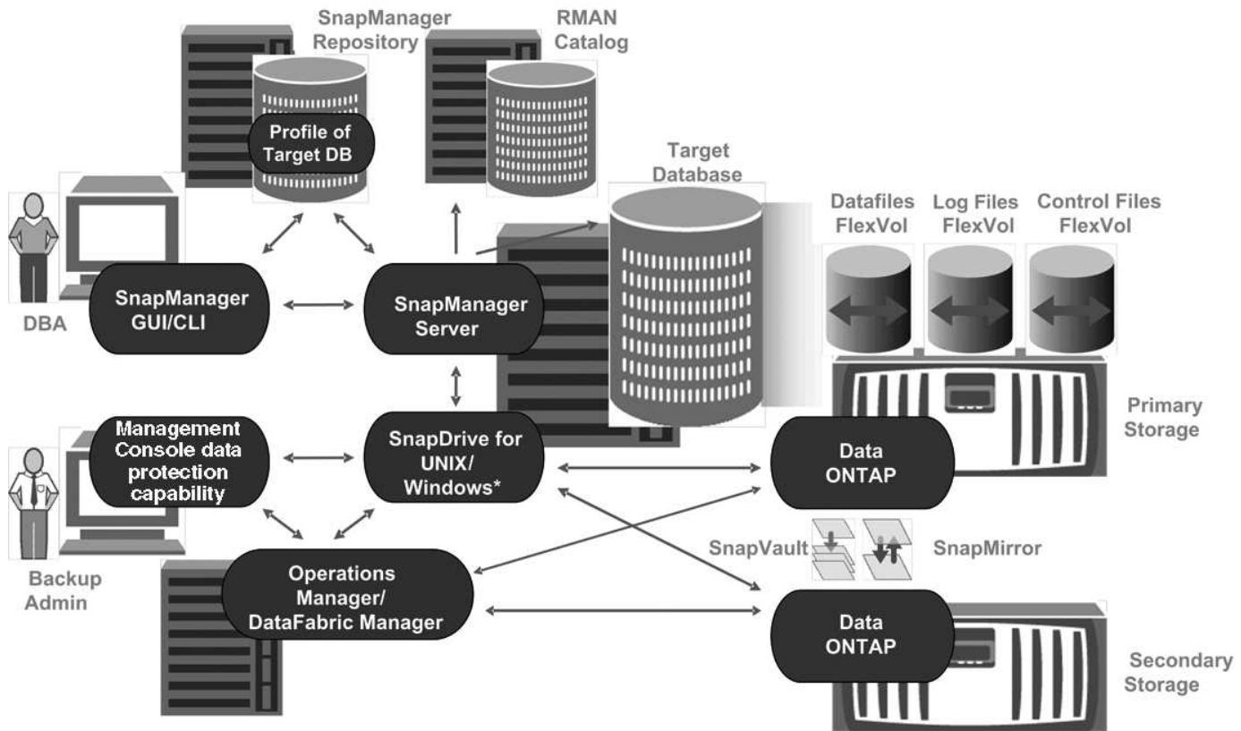
To manage the payroll database and support its local and secondary backup protection as illustrated in the previous graphic, the following deployment is used.
