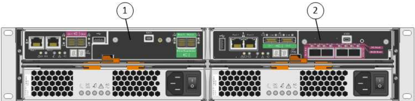
Model SG5612 2U: Rear view of the E2700 controller and E5600SG controller
