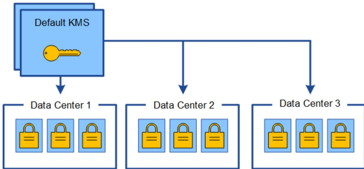
3. You decide to add a site-specific KMS for one site (Data Center 3 in the figure). However, because the appliance nodes are already encrypted, a validation error occurs when you attempt to save the configuration for the site-specific KMS. The error occurs because the site-specific KMS does not have the correct key to decrypt the nodes at that site.
