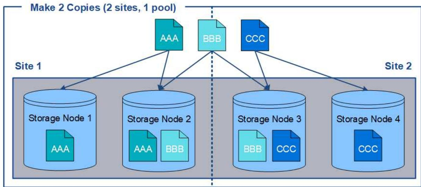
In contrast, this example illustrates how objects are stored when you use multiple storage pools. In the example, the ILM rule specifies that two replicated copies of each object be created, and that the copies be distributed to two storage pools. Each storage pool contains all Storage Nodes at one site. Because a copy of each object is stored at each site, object data is protected from site failure or inaccessibility.
