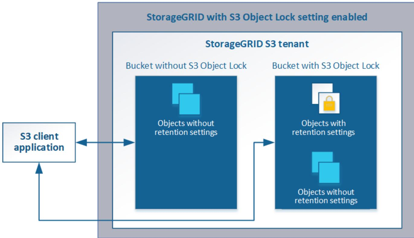
The StorageGRID S3 Object Lock feature provides a single retention mode that is equivalent to the Amazon S3 compliance mode. By default, a protected object version cannot be overwritten or deleted by any user. The StorageGRID S3 Object Lock feature does not support a governance mode, and it does not allow users with special permissions to bypass retention settings or to delete protected objects.
