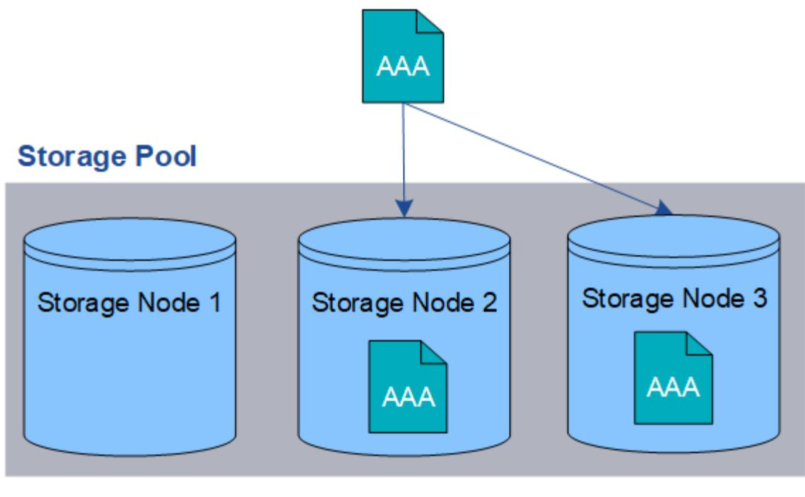
When StorageGRID matches objects to this rule, it creates two copies of the object, placing each copy on a different Storage Node in the storage pool. The two copies might be placed on any two of the three available Storage Nodes. In this case, the rule placed object copies on Storage Nodes 2 and 3. Because there are two copies, the object can be retrieved if any of the nodes in the storage pool fails.
