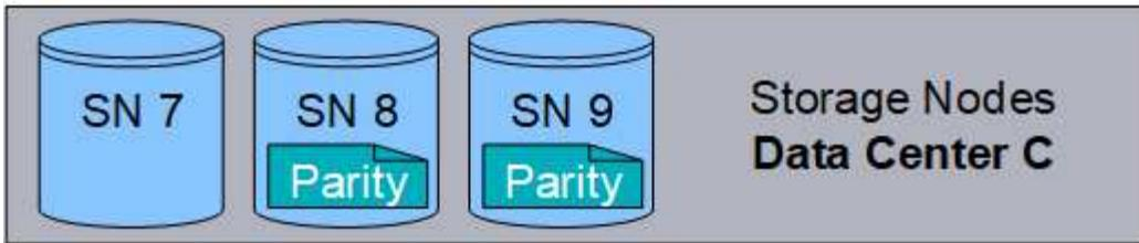
The 4+2 erasure-coding scheme requires a minimum of nine Storage Nodes, with three Storage Nodes at each of three different sites. An object can be retrieved as long as any four of the six fragments (data or parity) remain available. Up to two fragments can be lost without loss of the object data. If an entire data center site is lost, the object can still be retrieved or repaired, as long as all of the other fragments remain accessible.
