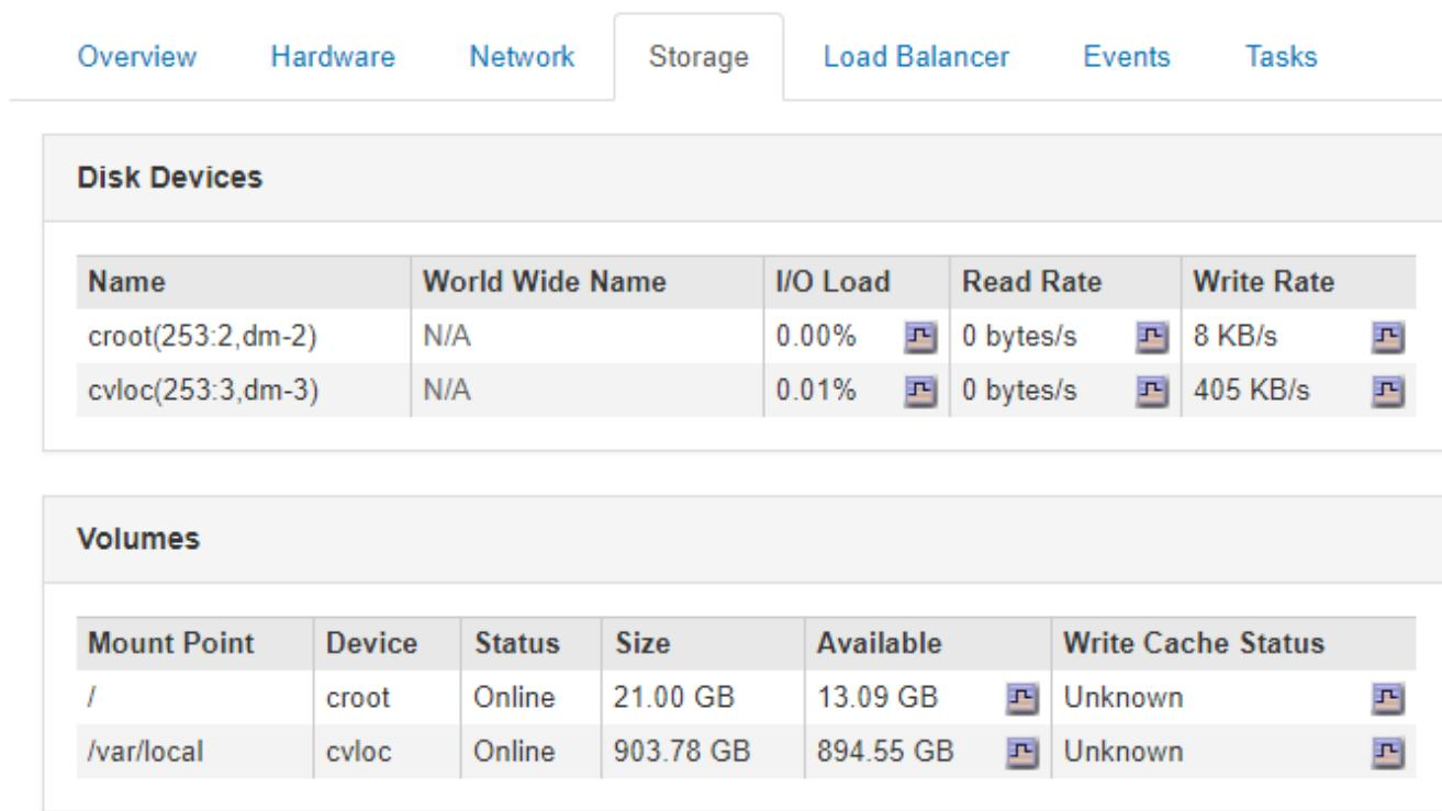
The screenshot shows the Storage tab selected in the top navigation bar. It displays two main sections: 'Disk Devices' and 'Volumes'.
