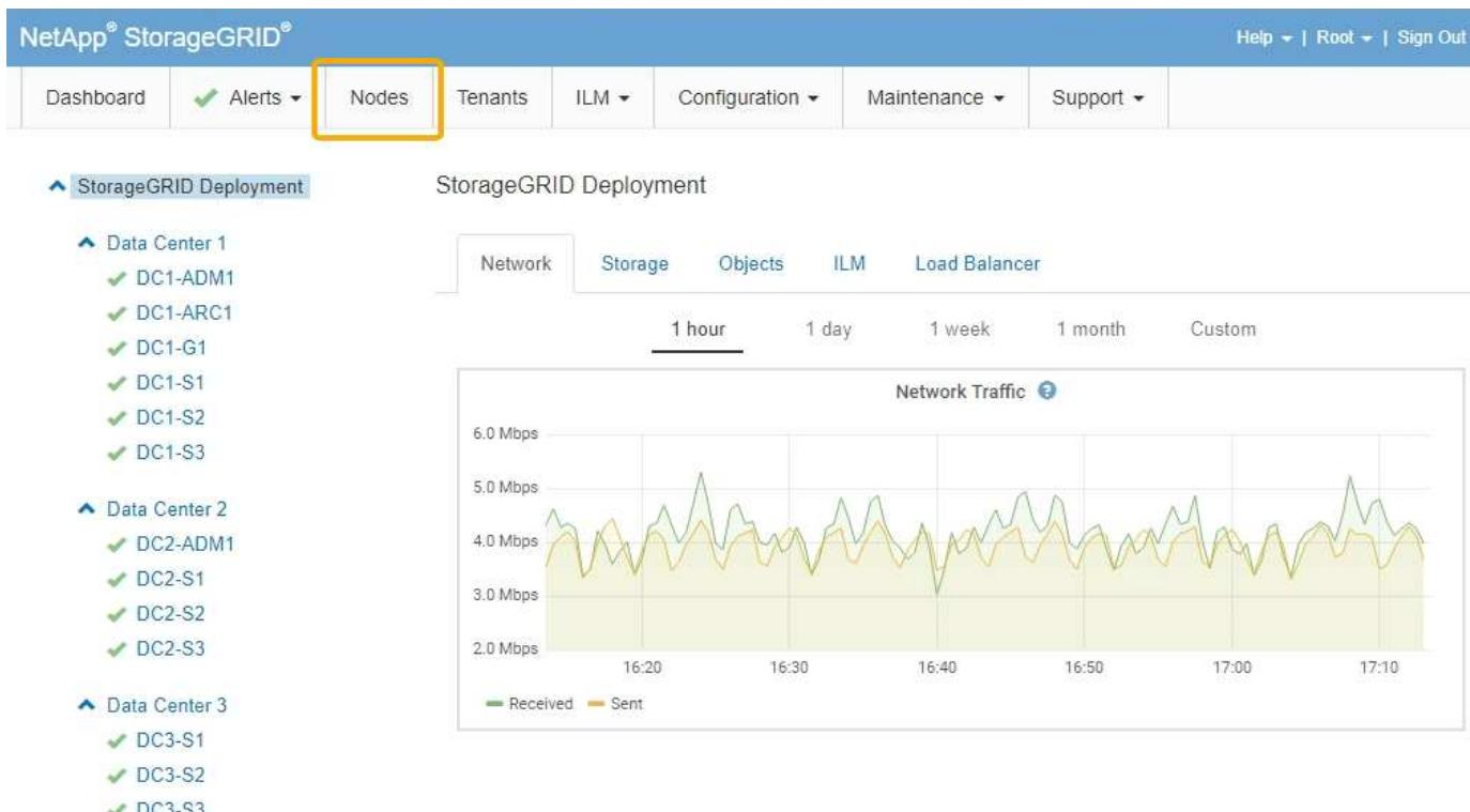
From the tree view on the left, you can see all the sites and all the nodes in your StorageGRID system. The icon for each node indicates if the node is connected or if there are any active alerts.
