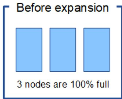
To expand the site in this example, it is recommended that you add three or more new Storage Nodes. StorageGRID requires three Storage Nodes for 2+1 erasure coding so that it can place the two data fragments and the one parity fragment on different nodes.
